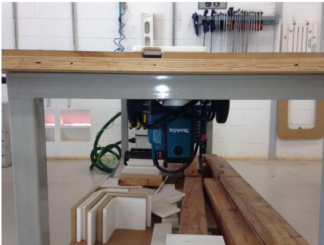
Figure 04: fixed router under working table to correct narrow pieces.
